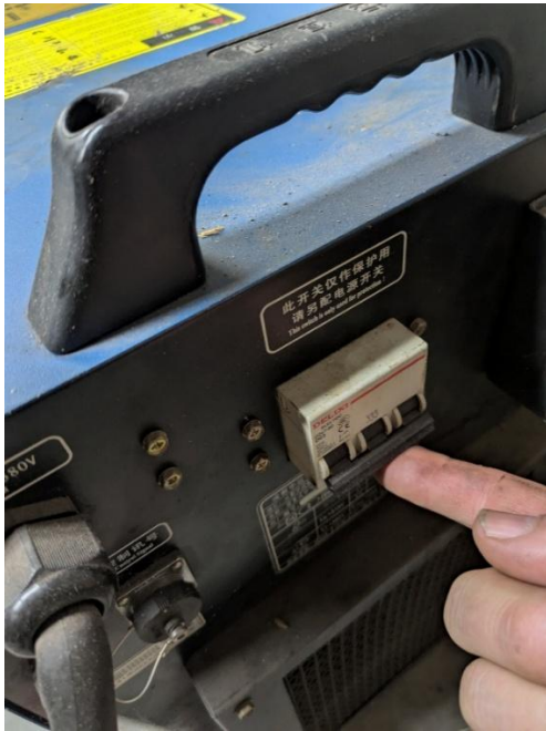
Turn on the Plasma Source. Flip the triple breaker up. Fans will run.
